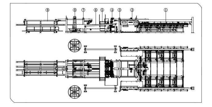
1.line wire tranferring and laying device 2.wire straightening and cutting machine
