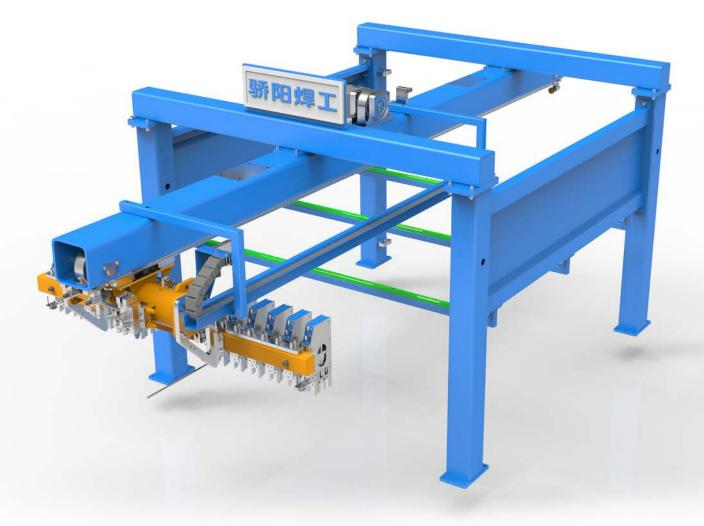
>With automatic robotic pneumnatic grippers for picking up line wires from the
