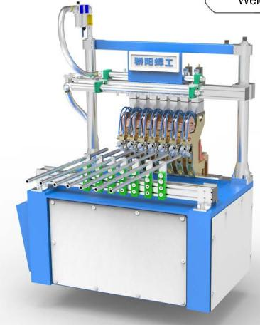
>Welding system adopst modular unit, and it will be more simple to adjust line wire spacing.
