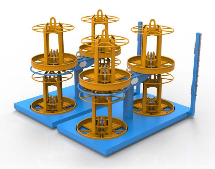
>The wire payoff adopt double layer which loading capacity is 500kg, save covering space.
