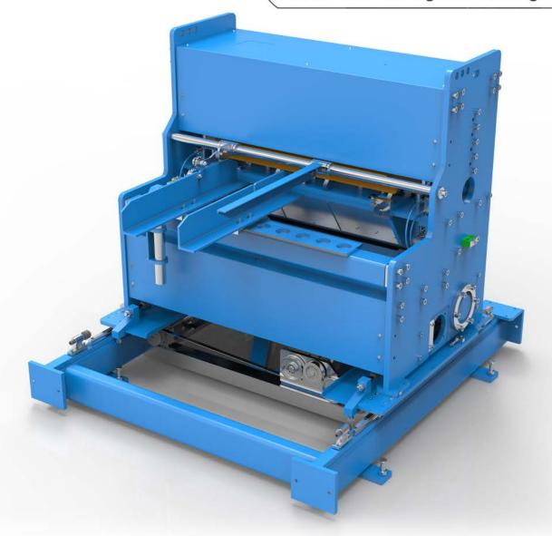
>The mesh cutting speed is 80 times /min and can realize the finished mesh without edges after cutting as requirements,no need to process manually anymore.
