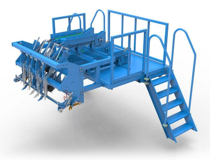
>The upper and lower hoppers adopt chain drive for feeding, and the storage capacity is 300kg.
