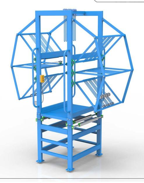
>The storage loop can reduce the resistance of pulling mesh, which can make the mesh size accurate and pulling mesh speed.
