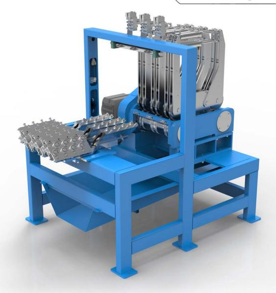
>It adopt two directions of 45° straightening, which will reduce the material prestress and the flatness of mesh will be ensured.
